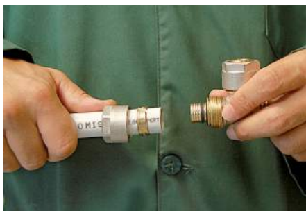
INSERTING THE FITTING / MONTAGGIO DEL RACCORDO / MONTAGE DES FITTINGS / INSERTION DU RACCORD
